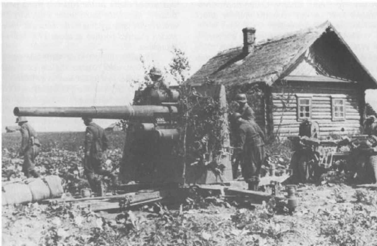
An 8.8 cm Flak 18 prepared to fire at ground targets on 4 August 1941. (GF)
