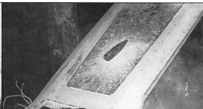
Above left, entry hole of 20mm shell in the nose cone of 138620. Above, windscreen strike position of bullet. (Grumman)
