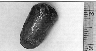
At left, bullet as found in the engine after the crash. Below, the bullet after its removal from the engine. (MFR via Meyer)
